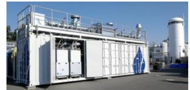
*Sunfire’s solid oxide cell electrolyzer*
