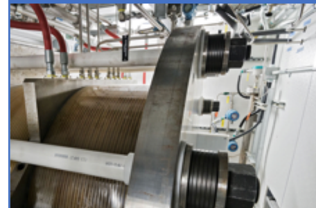
Electrolyser, used to split water into H and O 2 with electricity
